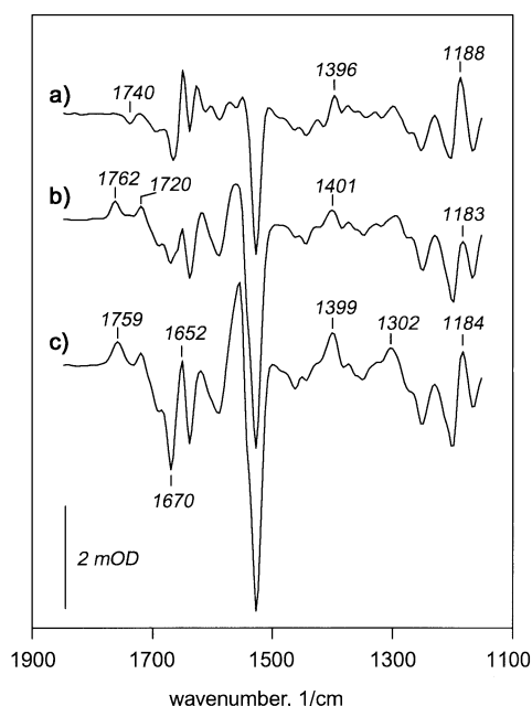
FIGURE 7: Amplitude spectra for E194D, from global fitting of FTIR difference spectra at pH 6.0. Trace a is extrapolated to the time before the \tau_2 process and corresponds to the L minus BR spectrum. Trace b is after the process described \tau_3 is completed (cf. Table 1) and corresponds to the M minus BR spectrum. Trace c is after the process described by \tau_6 is completed (cf. Table 1) and corresponds to the (M plus N) minus BR spectrum.
